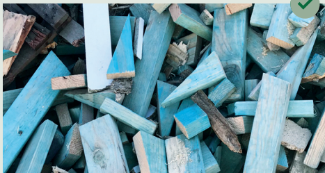
Bluepine (H2F) softwood offcuts and dockings Preservative code number indicates type of preservative used. Blue colour and H2F indicates envelope treatment.
