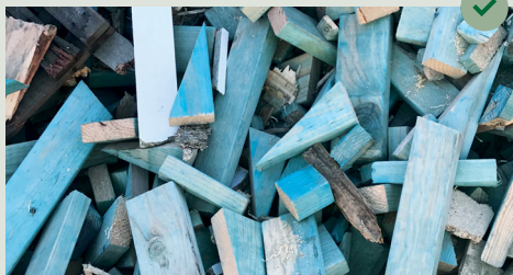
Bluepine (H2F) softwood offcuts and dockings Preservative code number indicates type of preservative used. Blue colour and H2F indicates envelope treatment.
