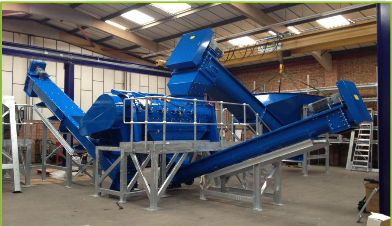
FIGURE 13 TYPICAL TURBO SEPARATOR USED FOR PROCESSING WASTE PLASTERBOARD
