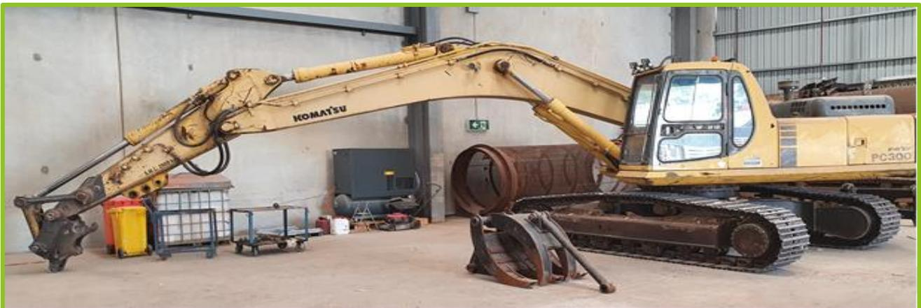
FIGURE 10 TYPICAL EXCAVATOR USED FOR MOVING AND MINIMISING WASTE WOOD AND PLASTERBOARD
