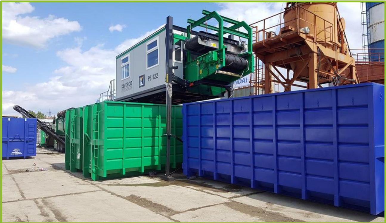
FIGURE 12 TYPICAL ELEVATED MANUAL PICKING LINE FOR SORTING OF WASTE WOOD/TIMBER
