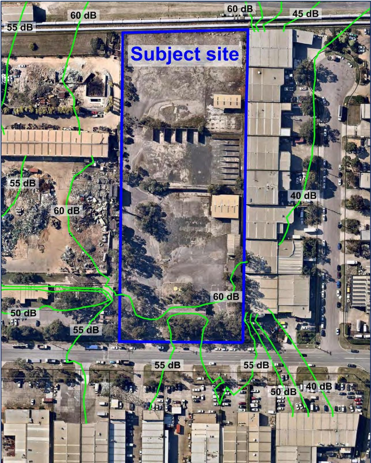
Figure 27: Near Field Noise Contours - Construction  $L_{Aeq,15minute}$  dB
