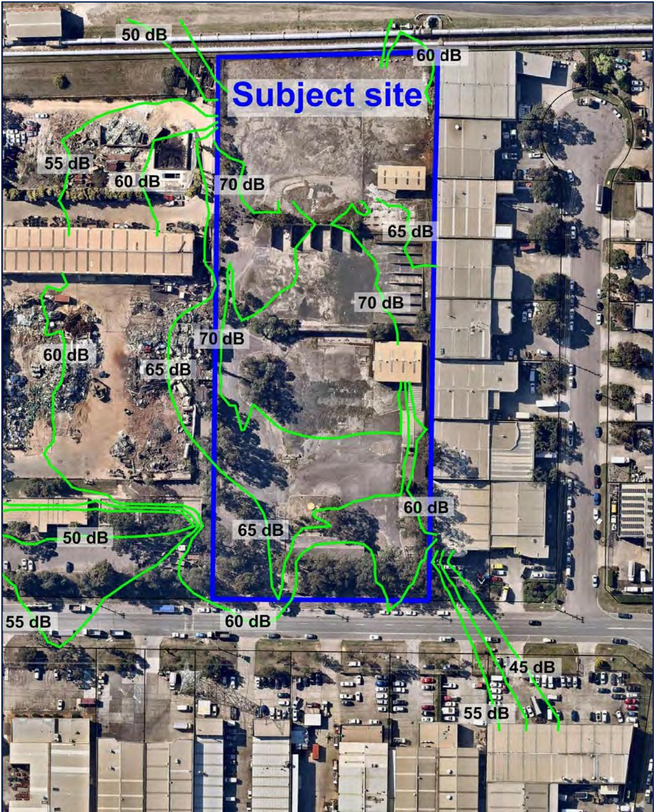
Figure 29: Near Field Noise Contours – Operational Morning Shoulder/Day Period  $L_{Aeq,15\text{minute}}$  dB
