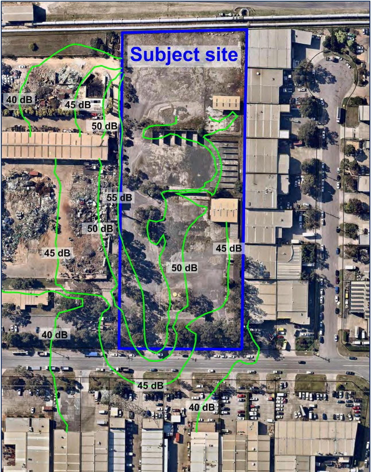
Figure 31: Near Field Noise Contours – Operational Evening/Night Period  $L_{Aeq,15\text{minute}}$  dB
