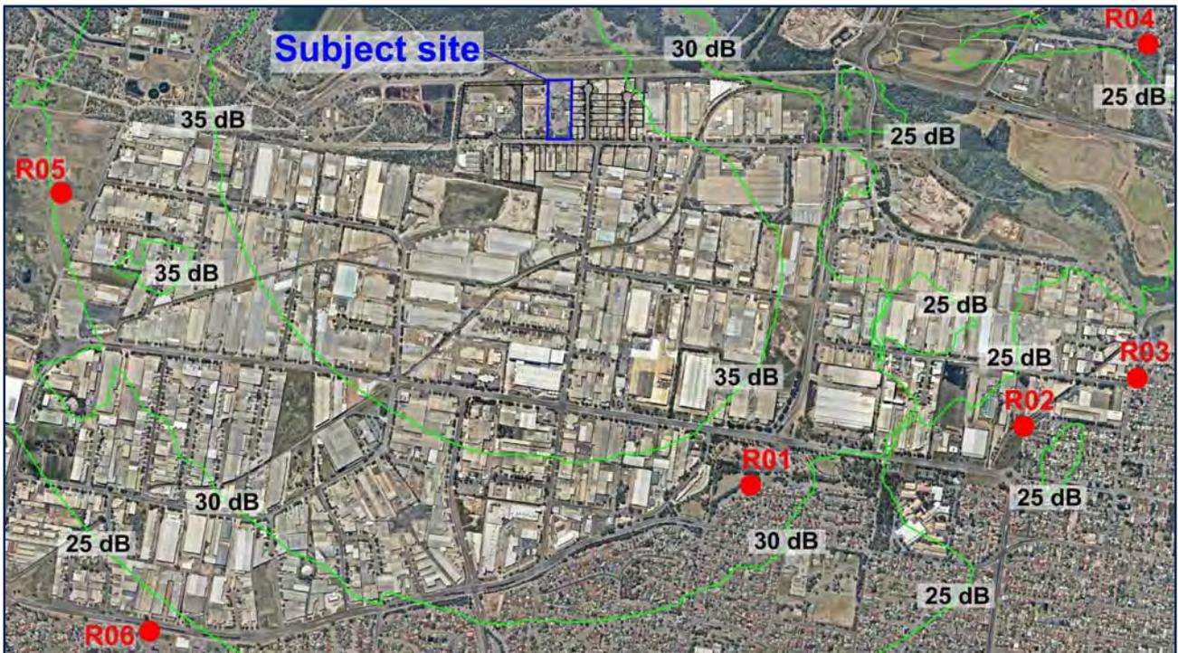
**Figure 30: Far Field Noise Contours – Operational Morning Shoulder/Day Period  $L_{Aeq,15\text{minute}}$  dB**
