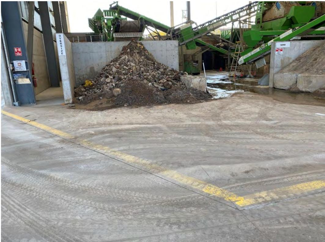
**Plate 12 – Oversize material stockpile showing bunding on shed floor**
