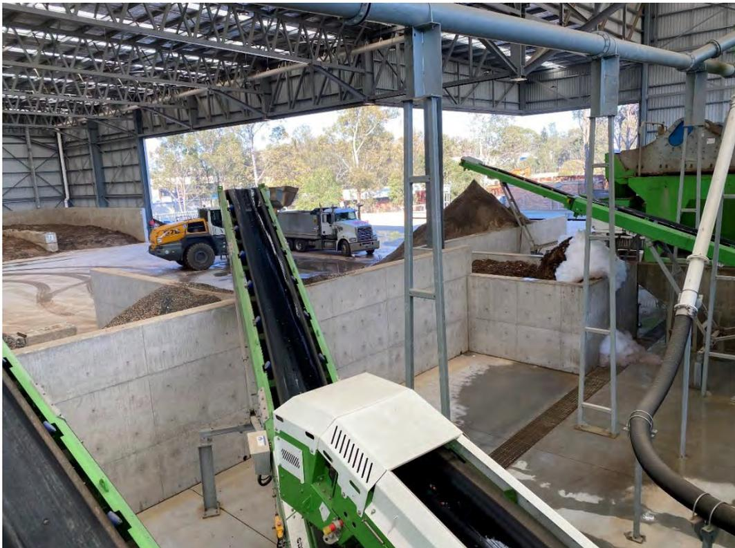
Plate 6 – Sand, organics and recovered aggregate conveyor belts
