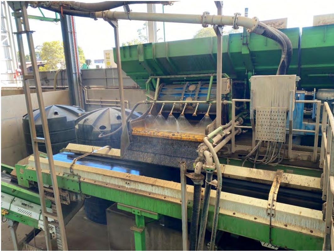
**Plate 7 – Recovered aggregate being sprayed and washed**
