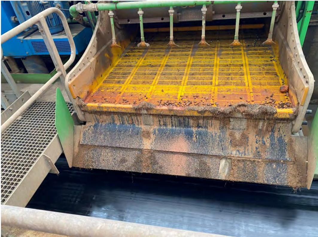
Plate 3 – Aggregate sprayers
