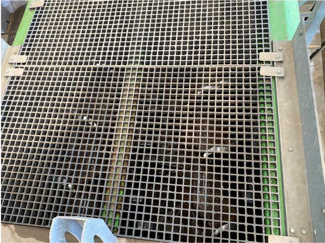
Plate 5 – Water tank in screener separating large solids
